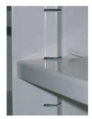
All Mailroom Sorters securely nest together using a unique, steel, 4-sided skirt. The horizontal sorting shelves on all Mailroom Sorters are removable and adjustable in 1 5/8" Increments. All shelves are punched with a tab on either side that can be lifted to keep shelf secured in place.
